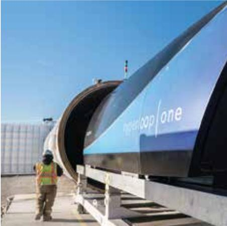
Hyperloop is a proposed transport mode that uses electrically propelled, magnetically levitated pods within near-vacuum tubes to carry goods or passengers at speeds of up to 760mph. By travelling within a sealed, low-pressure environment, and by 'floating' the vehicle above the track using the repulsion of two magnets rather than wheels, the pods travel free of air resistance and friction, and three times faster than conventional magnetic levitation (maglev) trains or high-speed rail (HSR).
